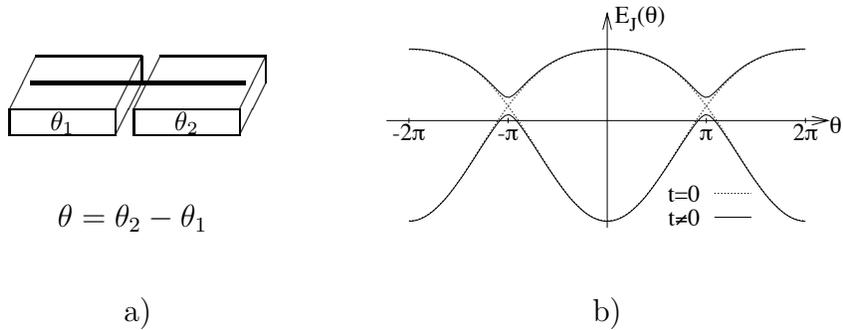
Figure 5: A Josephson junction made of quantum wire.
