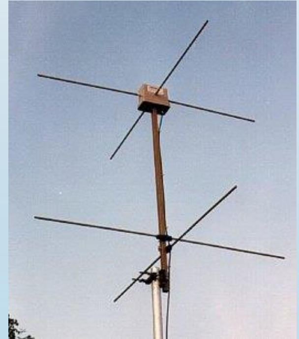
KX-137 VHF Satellite Antenna for polar orbiter satellites with built-in Preamplifier and High-Q-Filter.
