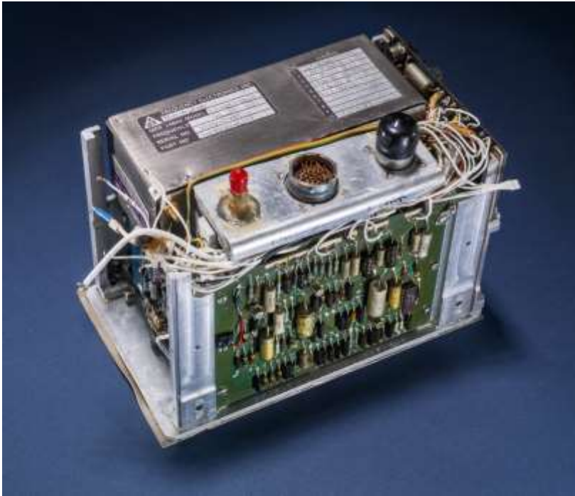
Caesium-133 atomic clock for GPS satellite (1970): 9 192 631 770 Hz
